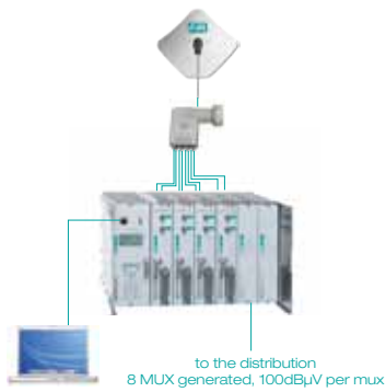
3DGFLEX - Using a msw to distribute signals to all receivers
